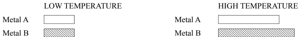
Next, I'll draw a thermostat. The two pieces of different metals in the thermostat are \*bent together. Now the metals are too hot. Then one metal gets longer than the other metal. So the two metals are bent more to the side of the shorter metal. The \*arm of the thermostat moves and it turns off the electricity. <sup>(5)</sup> Look at this picture.
